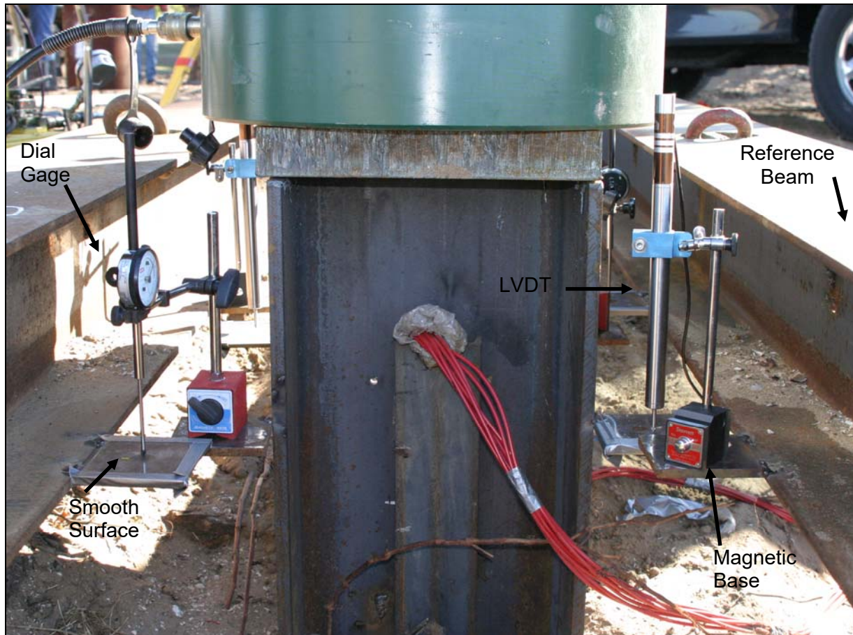
Figure 9-65. Load test movement monitoring components (FHWA, 2006a).
